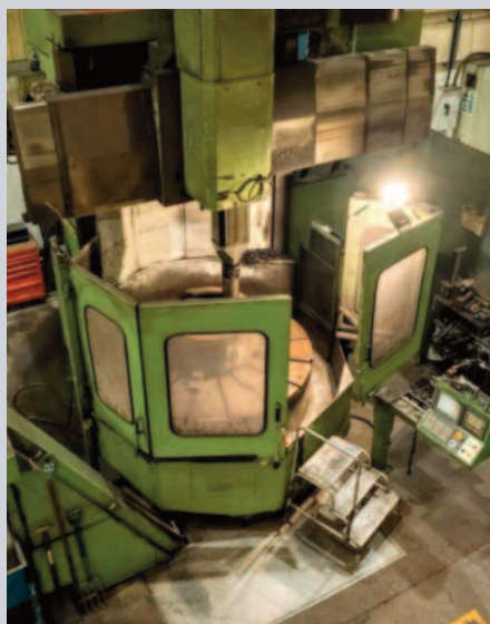
Schiess CNC Vertical boring
